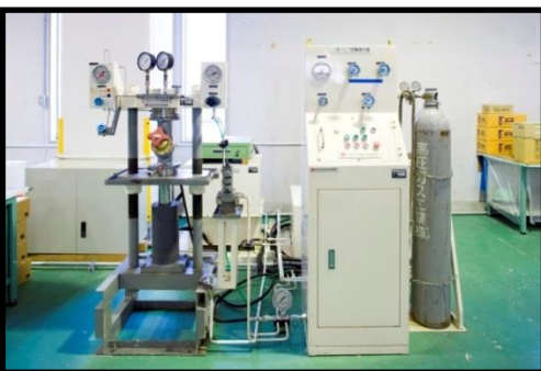
External Leakage Testing
